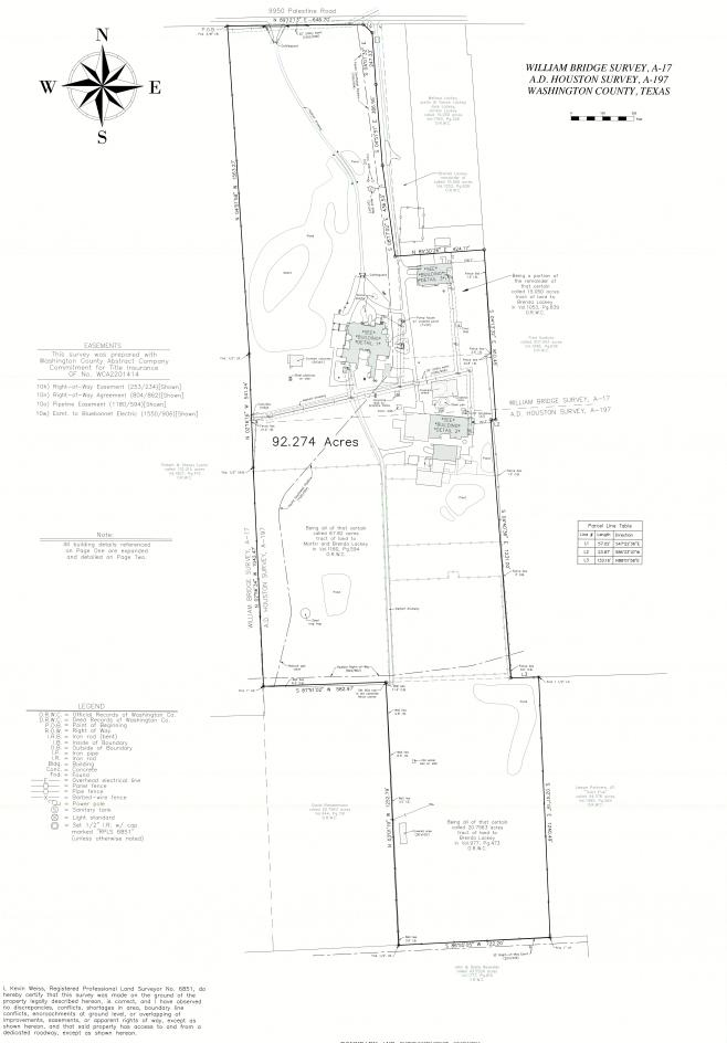
All bearings and distances are based on State Plane Coordinate System, Texas Central Zone, NAD 1983.
